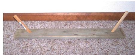
The base and the two wooden dowels angled and screwed into it.
